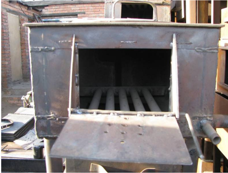
Photograph 6 - Low pressure boiler, note water pipes
